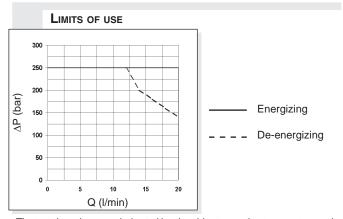
The tests have been carried out with solenoids at operating temperature and a voltage 10% less than rated voltage with a fluid temperature of 50  $^{\circ}$ C. The fluid used was a mineral oil with a viscosity of 46 mm²/s at 40 degrees C.
