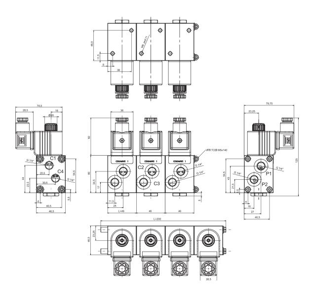
Tighten the screws to a torque of 5 Nm (0.5 Kgm) Fixing screws with material specifications min. 8.8
