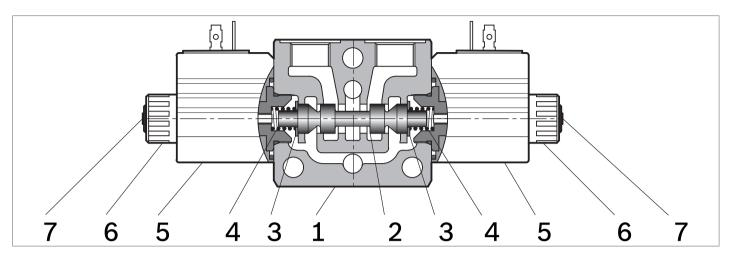
The sandwich plate design directional valve elements L8\_10... are compact direct operated solenoid valves which control the start, the stop and the direction of the oil flow. These elements basically consist of a stackable housing (1) with a control spool (2), one or two solenoids (5), and one or two return springs (4).
